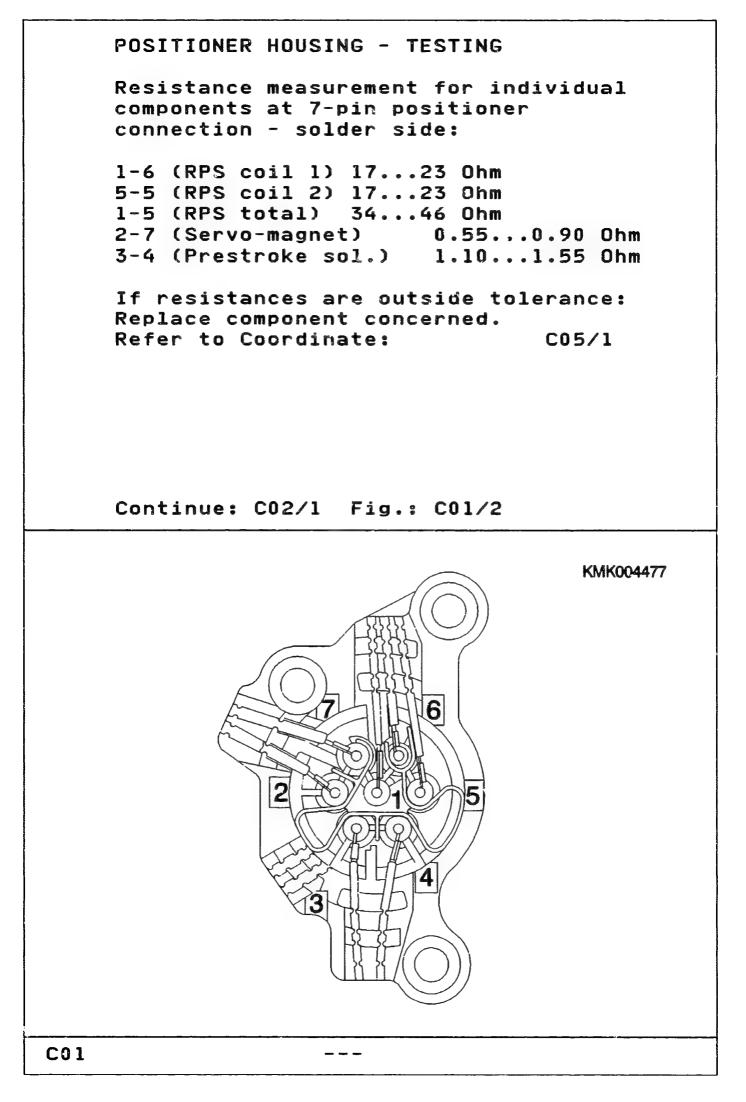
In the case of positioner version with cable bushing and overhung plug, check leads from plug to terminal board for continuity and mutual short circuit. Refer to following Coordinates for plug assignment. Test specifications: Continuity test: 0 Ohm. Mutual short circuit: infinity Ohm Note on short-circuit test: When mutually checking leads to a component, the value is not infinity Ohm, but rather in line with the coil resistance of the component.
